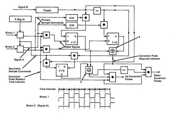
The problem: To design a circuit that generates correction signals to control the frequency of a voltage-controlled oscillator in a system used to acquire and track incoming signals over a wide range of frequencies.
