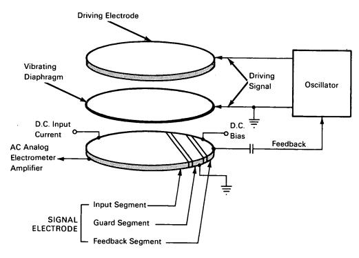
**The problem:** To provide regenerative feedback to an oscillator driving a dynamic capacitor in the input stage of an electrometer circuit. Prior art used a variable reluctance pickup having a single input electrode on the side of the vibrating diaphragm opposite the driving electrode. Difficulty has been experienced in providing sufficient feedback from the variable reluctance pickup and in sufficiently reducing its temperature coefficient.
