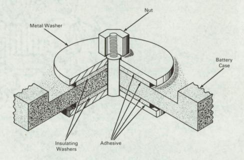
The problem: To reduce leakage through alkaline battery seals. Present seals frequently develop leaks or fail under reduced pressure because the adhesive fails. A plastic sealant such as epoxy resin may be applied to critical areas of a seal, but even such a sealant cannot withstand the erosive action of caustic electrolyte for prolonged periods.
