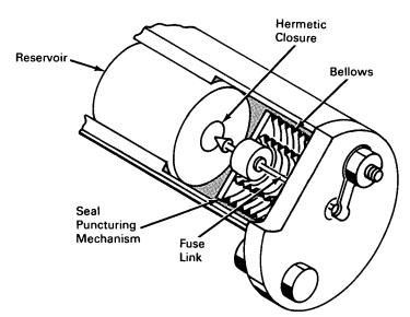
**The problem:** To provide a hermetically sealed closure with an emergency release that can be actuated by a remote sensor.
