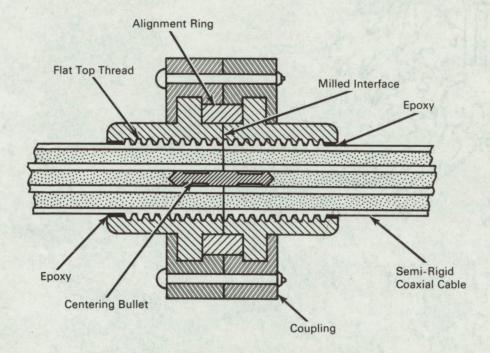
The problem: To design a connector, for flexible, semirigid, and rigid rf coaxial cables, that eliminates the possibility of secondary-emission discharge and provides low signal loss, low VSWR, lightweight construction, and good protection of the cable ends.
