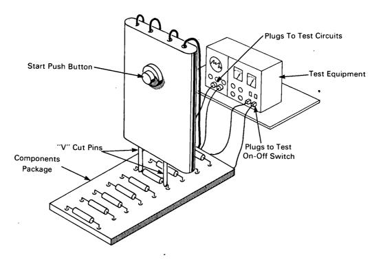
The problem: Testing of electronic components in volume has been a time consuming task involving unpackaging and repackaging for coded storage according to test results. Handling of small, sensitive components also results in a certain percent that must be discarded due to damage to leads, seals, etc.
