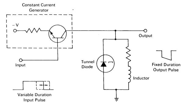
**The problem:** To generate an output pulse of fixed duration from a variable duration input pulse ranging from 50 to several hundred nanoseconds. Prior art differentiated the input pulse to obtain a trigger pulse to be applied to a monostable or blocking oscillator. This method requires complex circuitry that consumes a relatively large amount of power.
