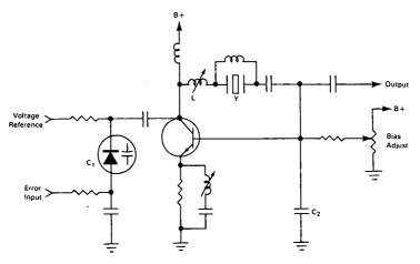
**The problem:** To design a voltage controlled oscillator (VCO) that can be easily adjusted for optimum performance. A conventional VCO, using crystal control and mutual inductance feedback coupling, requires a considerable amount of trial and error experimentation to select the best crystal and circuit parameters for stable operation and minimum phase noise.
