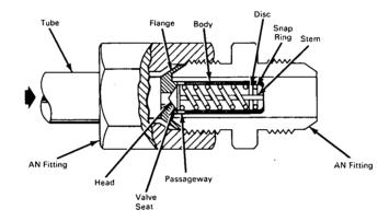
**The problem:** To design a compact all-metal check valve that can be used in standard AN fittings.
