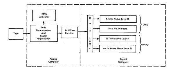
The problem: A complete space vehicle responds, during launch, to a variety of loadings, the study of which requires the outputs of many sensors. Analyzing these data graphically by hand introduces delays and human error factors. A rapid, accurate determination of probability distributions from the sensor outputs is needed.
