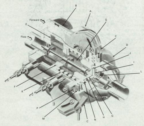
The problem: To develop a device which allows quick and safe uncoupling of plumbing during ground-to-vehicle transfer of cryogenic fluids and hazardous fluids such as fluorine.
