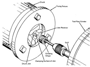
The problem: To properly position and rigidly hold lathe chuck jaws for refacing and truing of the clamping surfaces. The ideal method would have the jaws clamp a holding fixture during refacing in the same manner a workpiece is held. Fixtures used previously either did not hold the jaws accurately or could not be used on different size chucks.
