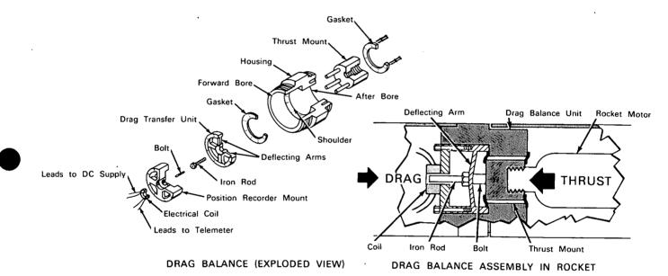
**The problem:** To measure the aerodynamic drag forces acting on a vehicle, such as a rocket, moving through the atmosphere.
