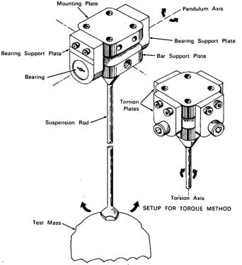
SETUP FOR PENDULUM METHOD
