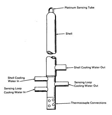
**The problem:** The design of an immersion temperature probe for use in a high-temperature, high-velocity gas stream poses problems that involve compromise between accuracy range and mechanical strength. Thermocouples cannot always be used near the limit of their melting points because aerodynamic loading, erosion, vibration, and fatigue reduce the practical limit well below this point.
