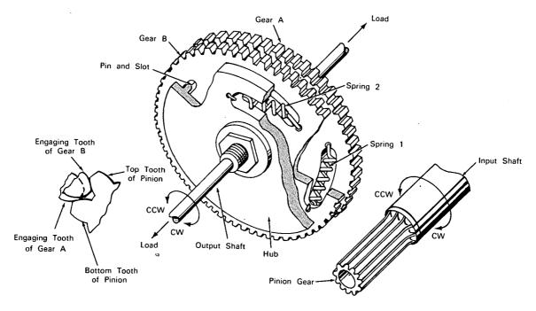
The problem: To maintain a constant output torque, free of backlash components, from a pulsating input torque.
