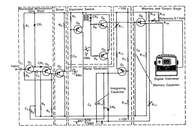
**The problem:** Analog cardiotachometers are inherently nonlinear and do not respond with sufficient speed to indicate rapid changes in heartbeat rate. Those digital cardiotachometers that are capable of measuring heartbeat rate on a beat-by-beat basis are generally complex and costly.
