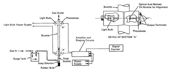
The problem: Calibrating flowmeters used for measuring low gas-flow rates (60 to 1000 milliliters per minute).
