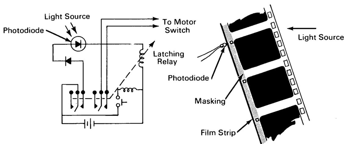
**The problem:** Automatically positioning individual frames on a strip of photographic film in a projector, viewer, or an enlarger.
