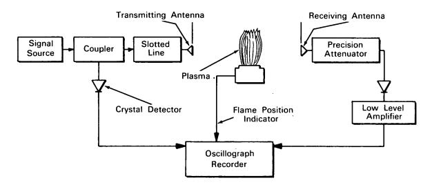
The problem: To obtain good spatial resolution in the measurement of plasma electron density and temperature distribution. This cannot be done using metallic probes because of: (1) the disturbance introduced into the plasma by the insertion of the probe; and (2) the effect that the plasma has on the probe.
