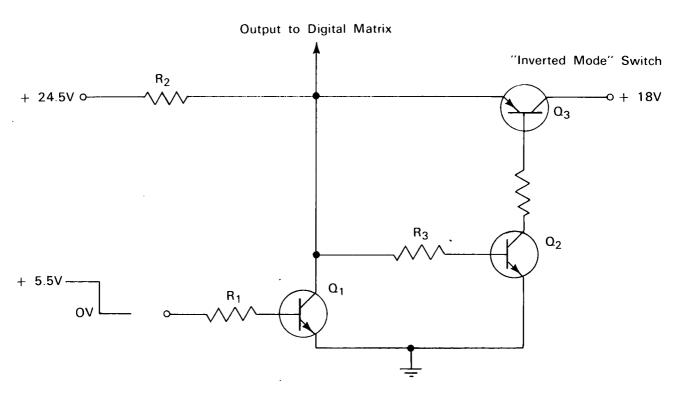
The problem: To apply two accurately clamped voltage levels (+18 or 0 volts) to the input of a digital-to-analog resistive matrix that binarily develops a deflection staircase.
