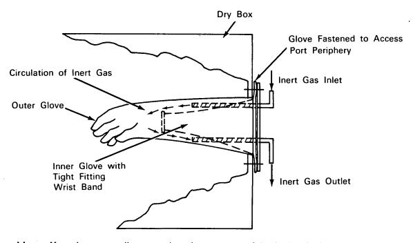
The problem: Hazardous or easily contaminated materials may be safely handled within a dry box fitted with rubber gloves for access. However, the inert atmosphere in the dry box may be contaminated by leakage of undesirable gases, such as water vapor and air, through the glove material.
