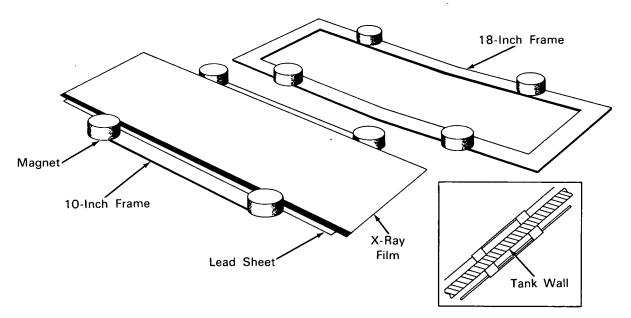
The problem: Inspections of welds by X-ray requires that the X-ray film be placed against the weld at the point to be inspected. In the case of large aluminum structures such as those used for space vehicle fuel and oxidizer tanks, placement of the film is difficult and frequently requires a man to enter the tank and tape the film in place.
