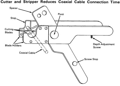
**The problem:** To prepare coaxial cable quickly and accurately for attachment of connectors. Stripping the insulation and shielding with a knife takes about three minutes per connection and requires a degree of skill.
