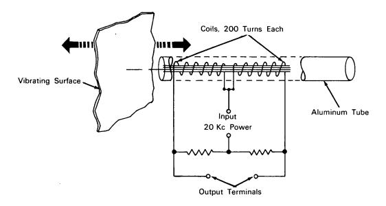
**The problem:** Measuring the surface displacements of nonferrous metal panels subjected to vibration or flutter such as produced by high-velocity winds. The transducer to be used for the measurements must not be placed in physical contact with any portion of the test panel.
