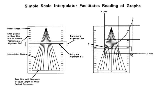
**The problem:** Providing a simple device to facilitate accurate and rapid reading of the coordinates of points on graphs plotted on relatively coarse rectangular grids.
