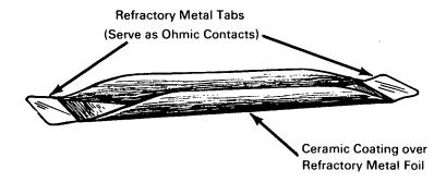
The problem: Providing an improved boat to be used as a container for metals or other inorganic materials that are to be evaporated in a vacuum furnace or evaporator. The boat must have good thermal conductivity, be physically strong, and chemically inert to the evaporants. Metal forms, twisted wire filaments, and ceramic crucibles which have been used as boats do not meet all of these requirements.
