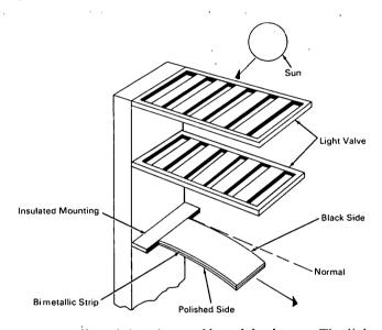
The problem: Many systems are affected by the presence of solar radiation. In those systems adversely affected by such radiation beyond a certain level, it is necessary to adjust or shield equipment as the relative position of the sun changes. The amount of heat and light energy received by an area is a function of the angle of incidence of the sun's rays on that area. A simple and reliable device is needed to provide control actuations as a function of solar incidence.
