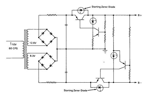
**The problem:** Power supplies using high-quality silicon transistors as variable impedance regulators require an initial starting current supply because these silicon transistors have exceedingly small leakage current. Previous starting techniques have been very complex and expensive.
