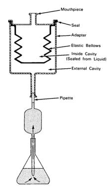
**The problem:** Protecting the mouth of a laboratory technician from harmful liquids, such as cyanide solutions, acids, alkalis, dyes, and bacteriological solutions, drawn up in standard pipettes through suction applied by the mouth.
