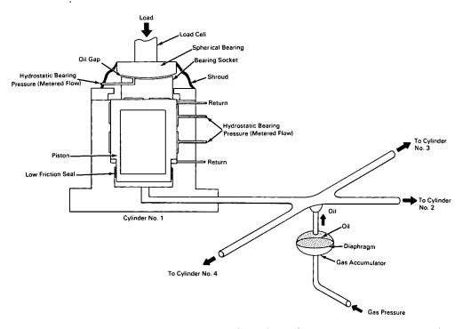
The problem: Providing a nonresonant support that will allow six degrees of freedom of motion of a large structure subjected to vibration testing. A primary purpose of the support is to enable the accurate determination of vibration frequencies and longitudinal mode shapes of large rocket systems.
