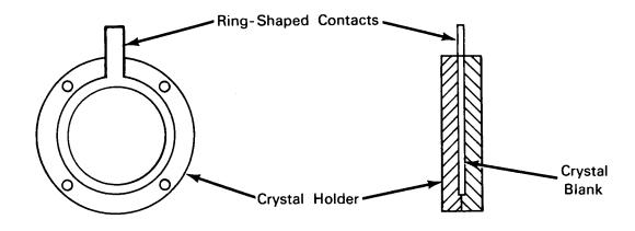
**The problem:** Piezoelectric crystals are used as the frequency determining elements in most electronic communication and computer equipment. Since mechanical stress of these crystals produces electrical potential changes on their surface, they must be protected from impact and vibration to assure reliable operation. The problem of mounting these crystals becomes acute when they are operated in electronic equipment which undergoes high accelerations and impacts.
