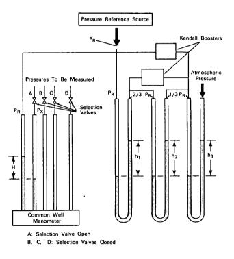
**The problem:** Measuring high fluid pressures by means of manometers. In situations where high pressures occur, an inordinately long column of liquid and tube would be required in a conventional manometer. Liquid blowout could also occur from the open end of such a manometer during pressure surges.
