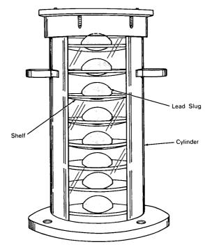
**The problem:** The suppression of response of structures to vibratory forces by addition of damping has in the past been difficult to achieve in a controlled manner. Previous methods have involved variation of tension in joints of the structure, wiring the structure to a dash/pot damper, and, in certain applications, coating the structure with an energy-absorbing material. All of these methods have exhibited deficiencies in applications where precise regulation of damping is of importance.
