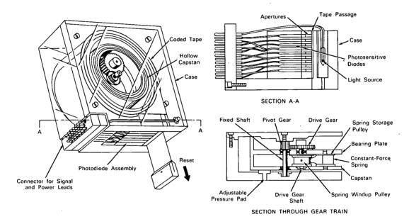
**The problem:** Facilitating storage and repetitive reading of short-program coded tape.
