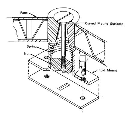
The problem: Provide flexible yet secure attachment of wind-tunnel research model skin sections. Thermal expansion of skin sections rigidly fastened to supporting structures produces stress concentrations which often cause the skin to rupture or buckle.
