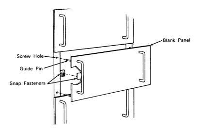
The problem: Quick fastening and unfastening of electronic assembly rack blank panels. The conventional method, requiring alignment of the panels and the use of screws to fasten them to the rack, is slow and awkward. Considerable time can be lost in removing screws when immediate access to the interior of the rack is required during operation of the electronic units.
