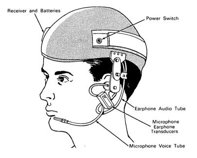
**The problem:** To provide communications by portable two-way radio under circumstances which require the wearing of a safety helmet. To date, safety helmets incorporating self-contained transceivers have been unwieldy and heavy, often with protruding components. Two-way radio components were mounted inside the helmet with only the webbing to prevent them from contacting the skull.
