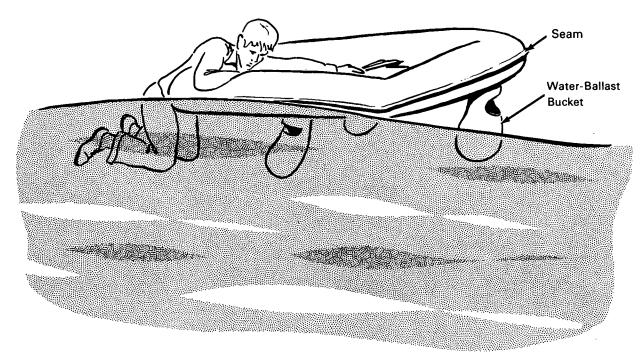
The problem: An improved inflatable liferaft for emergency use on the sea was required for Project Mercury. It was desired that the raft be lighter, more compact in packaged and inflated forms, more stable, and easier to manufacture than earlier models.
