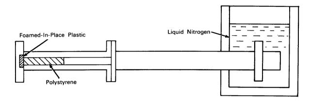
The problem: Microwave waveguide windows normally consist of thin dielectric membranes inserted between waveguide flanges. In microwave applications requiring the use of a cryogenically cooled waveguide, these windows receive condensation from the atmosphere and require special venting and sealing techniques.
