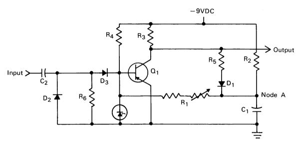
The problem: Design an improved monostable multivibrator (MSMV). Present devices fail to meet ideal operating characteristics in that output voltage rise time is greater than desired; the time period from quasi-stable to stable state is not constant; and available duty cycle time is typically only 65% of operating time.
