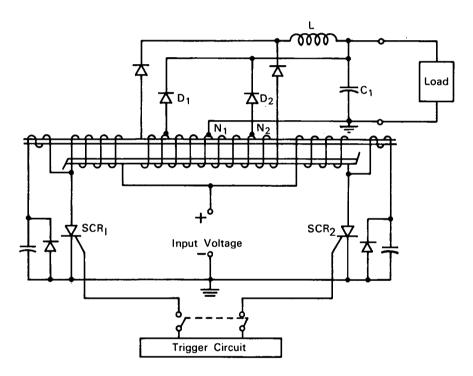
**The problem:** To eliminate starting difficulties encountered in d-c to d-c converters that employ an SCR (silicon controlled rectifier) d-c to a-c inversion stage with large output-filter capacitances.
