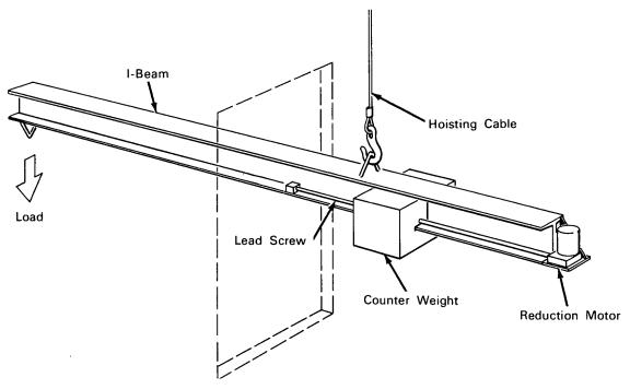
The problem: Moving heavy machine parts or other loads when they are located under an overhang so that a crane cannot be used directly. A similar problem is encountered in moving machinery or heavy parts through windows or doorways.
