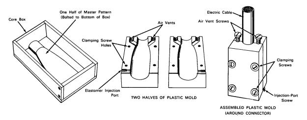
**The problem:** Providing an inexpensive method of fabricating a mold used for encapsulating or sheathing electrical cable connectors with an elastomer. The cost of fabricating molds by conventional methods can be an appreciable factor when it is required to encapsulate small quantities of connectors of different configurations.
