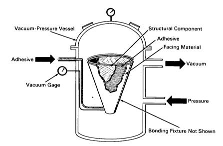
The problem: The advent of epoxy resins has greatly increased the use of adhesive bonding as a structural technique. In structural applications involving high vibrational, impact, or heat environments, voids or air pockets in the bond line introduce weaknesses that endanger the integrity of the bond.
