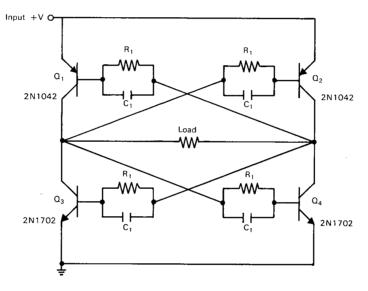
**The problem:** To develop a compact square-wave oscillator that will operate with high efficiency at relatively high power levels.
