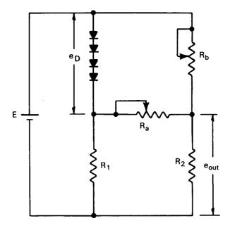
**The problem:** To design a simple circuit giving an adjustable output voltage that varies linearly with temperature.
