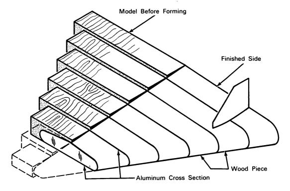
The problem: Reducing the time required to make an accurate, true-to-scale model needed for research testing or industrial needs. Testing of aircraft, ships, or rockets often requires quick construction of an accurate model in order to complete an experiment or cross-check research findings.
