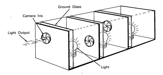
The problem: Development wide-range variable-intensity light source of constant color characteristics, that can be used for the testing and calibration of photo-multiplier tubes.
