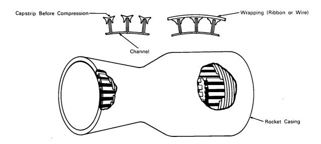
The problem: Increasing the strength and heattransfer characteristics of lightweight rocket motor casings that employ channels for regenerative cooling.
